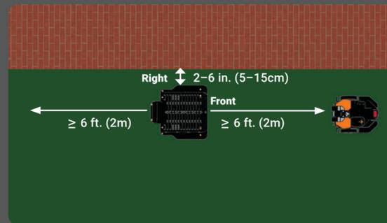
**\*IMPORTANT\*** Vision setup cannot be completed unless the charging station is correctly installed. Make sure Vision properly returns to the base after its first run (see Step 8). If it has trouble, make adjustments until it successfully returns.
